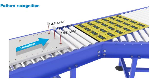
The pattern recognition function is used to verify if a manufactured part has all the e.g. holes or taps as expected and that the parts are made according to the specification.
